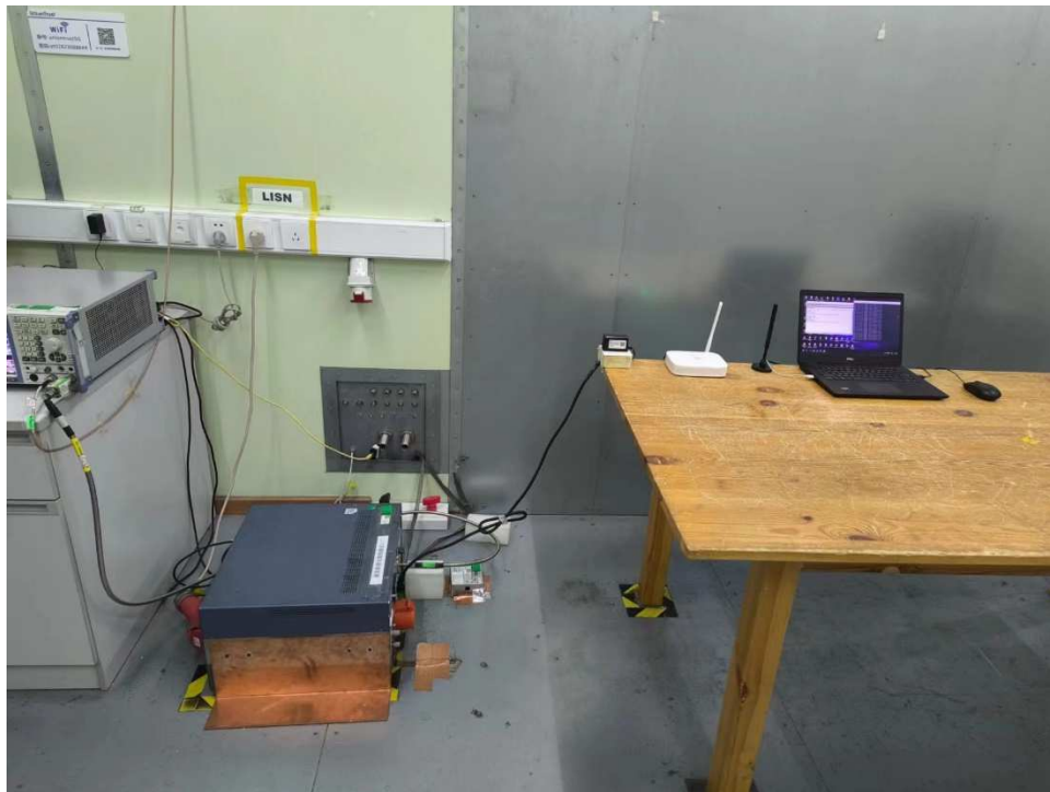
Photograph 1: Set-up for Conducted Emissions, AC Mains
