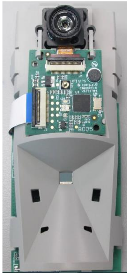
Photograph No.1 Wireless Motion detector with integrated camera PCB Camera
