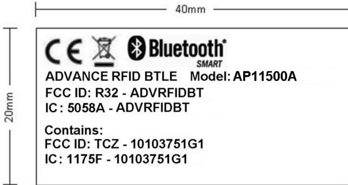
Figure 2. General layout and dimensions appearing on the ADV label.
