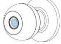
After unlocking the lock, shortly press the deadlock button for 3 times within 5s to enter into fingerprint's setting step. It will automatically exit from this function setting mode with 8s if no operation performed.
