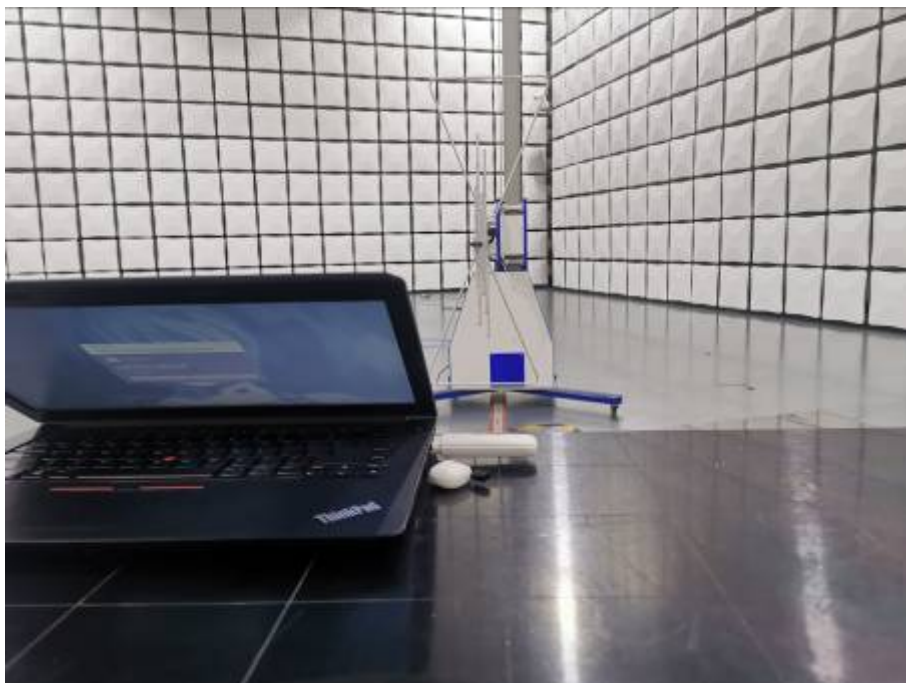
Radiated Emissions Test Setup (30-1000MHz)
