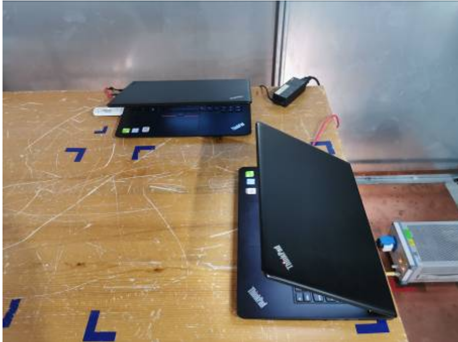
Conducted Emissions Test Setup
