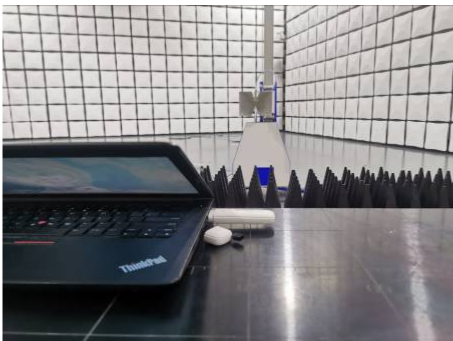
Radiated Emissions Test Setup (above1GHz)
