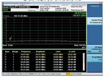
30MHz – 869MHz Channel Frequency 871.5+877.5MHz, QPSK/16QAM, 5+5MHz BW, TX2
