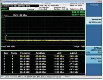
1GHz – 1.3GHz Channel Frequency 871MHz, 64QAM, TX1
