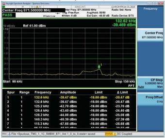
30MHz – 869MHz Channel Frequency 871MHz, 64QAM, TX1
