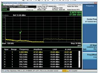
894MHz – 1GHz Channel Frequency 874+885MHz, QPSK/16QAM, 10+10MHz BW, TX1
