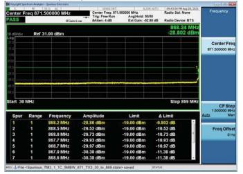
150kHz – 30MHz Channel Frequency 871.5MHz, 64QAM, 10MHz BW, TX3
