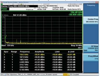
894MHz – 1GHz Channel Frequency 885MHz, 256QAM
