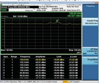
150kHz – 30MHz Channel Frequency 885MHz, 64QAM
