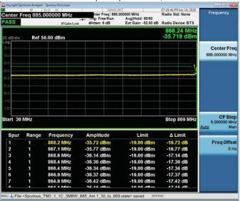
1GHz – 1.3GHz Channel Frequency 885MHz, 64QAM
