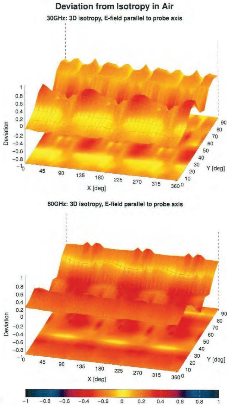
Probe isotropy for  $E_{tot}$ : probe rotated  $\phi = 0^\circ$  to  $360^\circ$ , tilted from field propagation direction  $\vec{k}$
