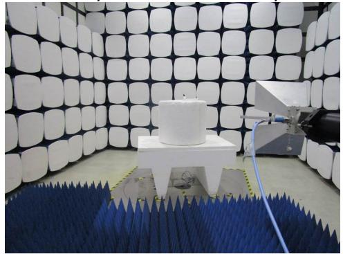
1.3 Radiated Spurious Emissions Test Setup
