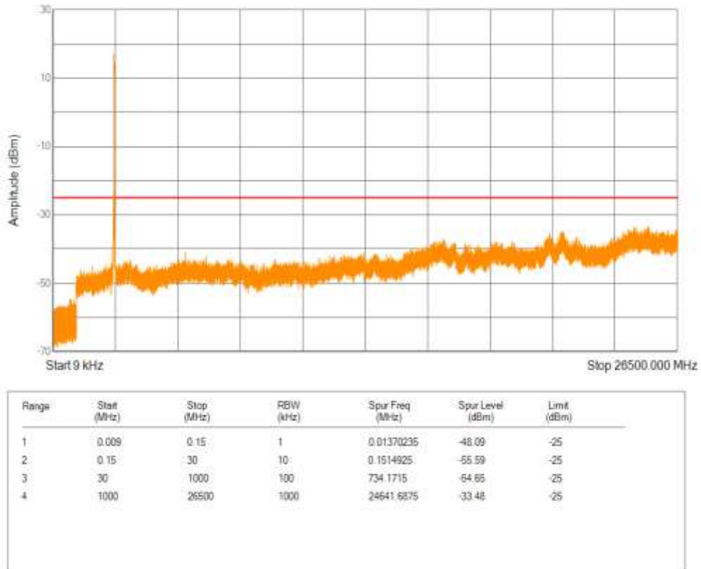
Band41(2555-2655) QPSK BW=20MHz Channel=41140 RB Size=100 Position=#0
