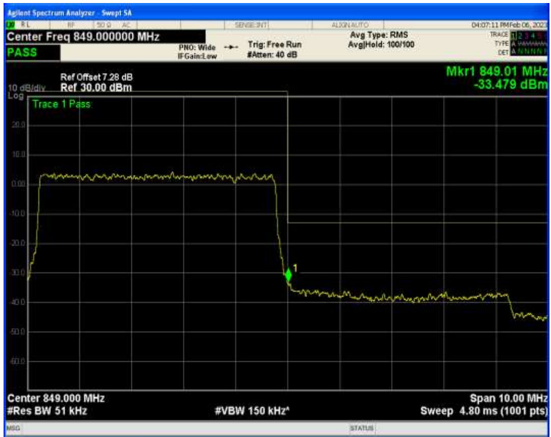
Band7 16QAM BW=10MHz Channel=20800 RB Size=50 Position=#0
