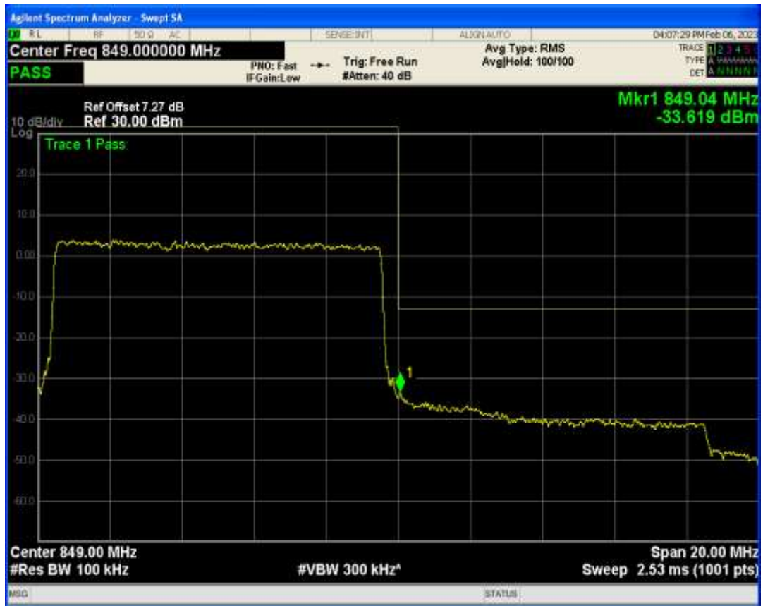
Band5 QPSK BW=3MHz Channel=20415 RB Size=15 Position=#0
