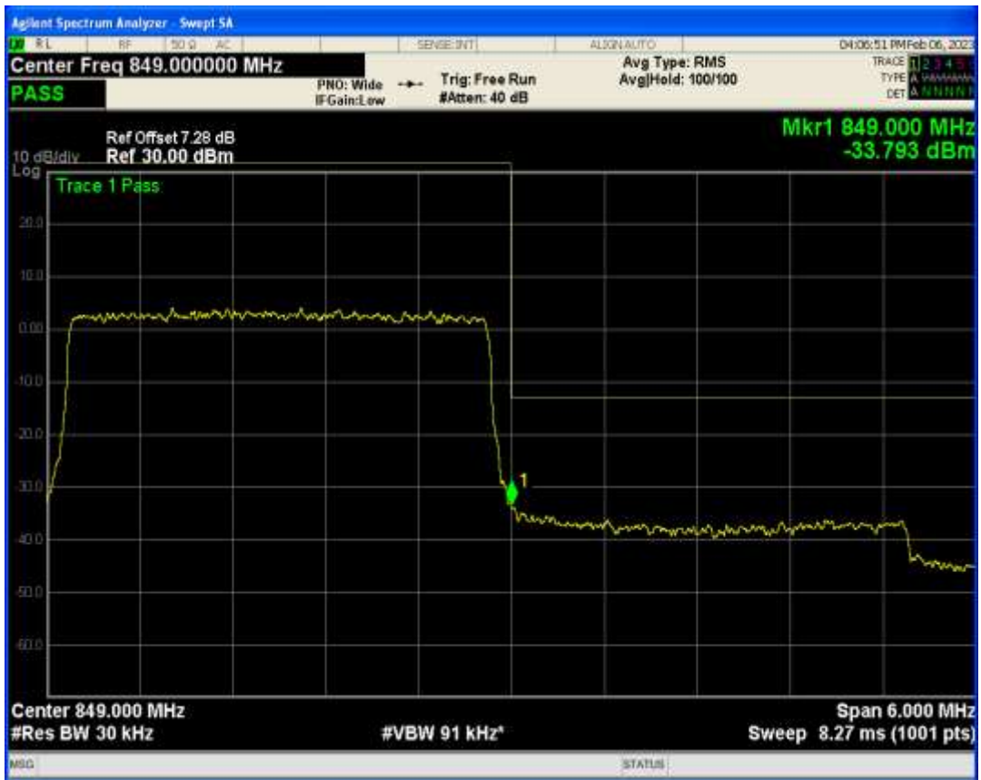
Band5 QPSK BW=5MHz Channel=20425 RB Size=25 Position=#0
