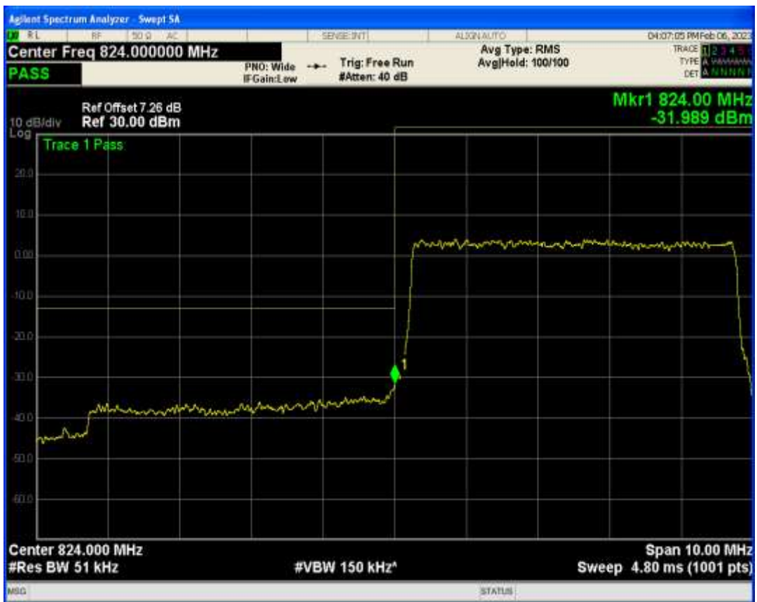
Band5 QPSK BW=5MHz Channel=20625 RB Size=25 Position=#0
