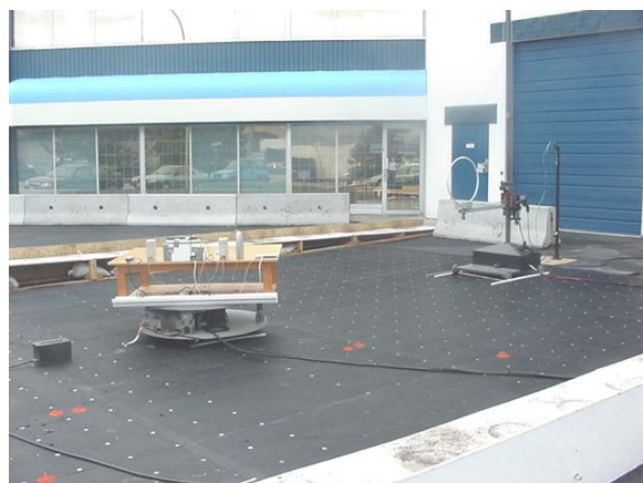
Photograph E-3 - 3115 Horn (1G - 2G) @ 3 m
