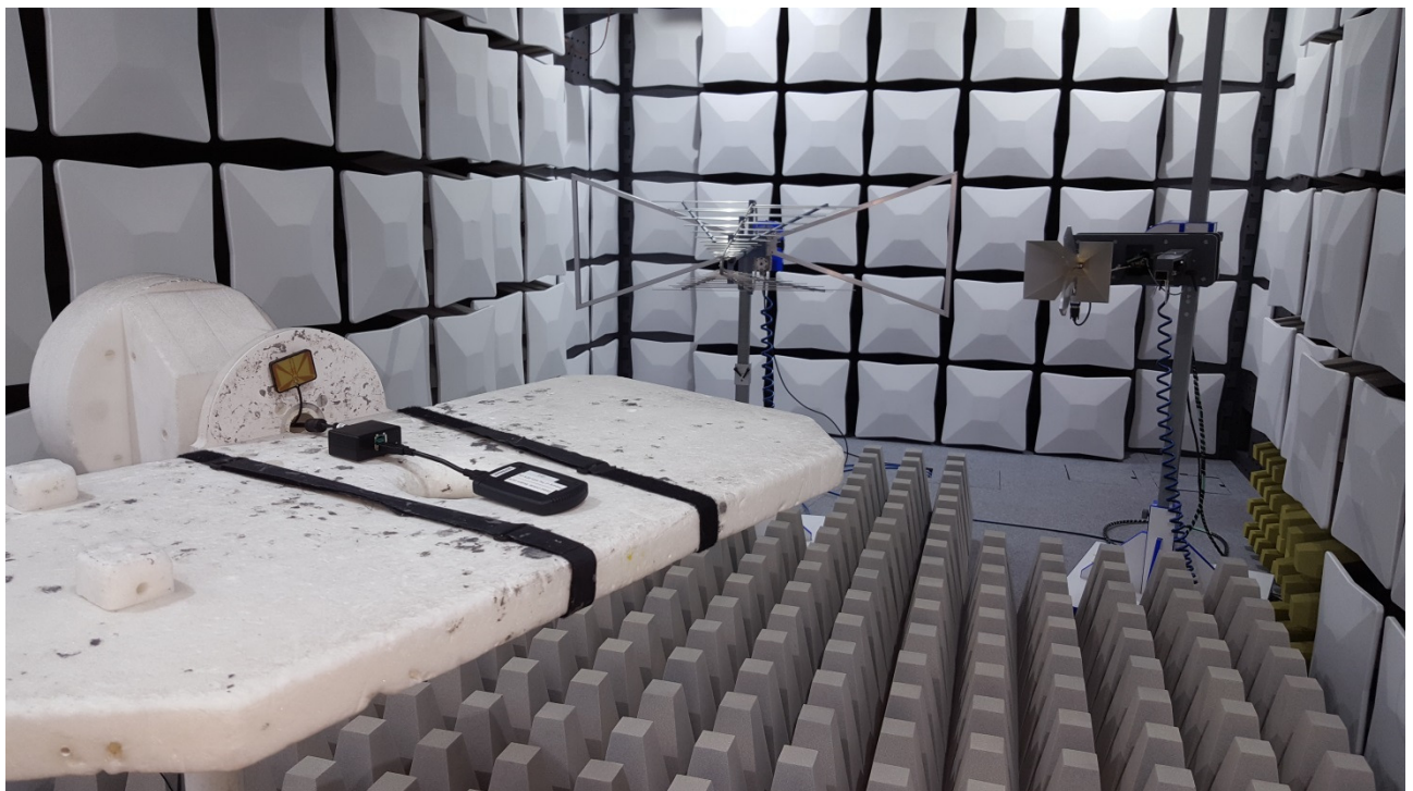
Photo 4: Test setup for radiated measurements in fully-anechoic chamber above 1 GHz
