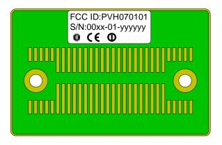
An auxiliary label will be provided for systems using the module where the original label not will be visible when the module is installed.
