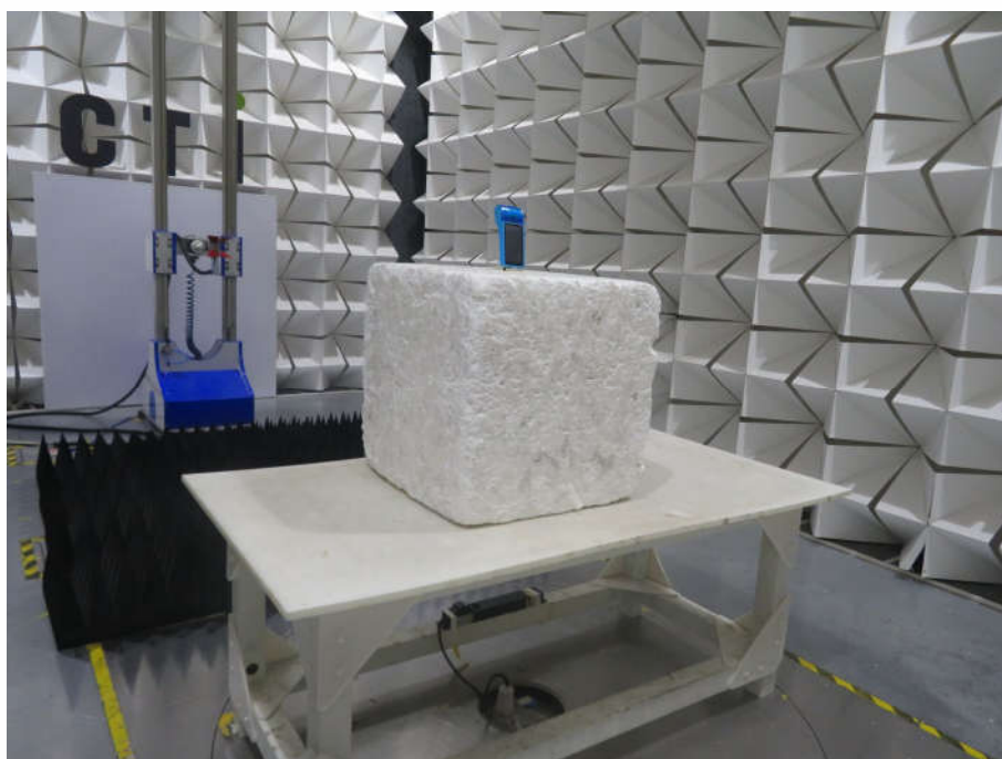
Radiated spurious emission Test Setup-3(Above 1G)
