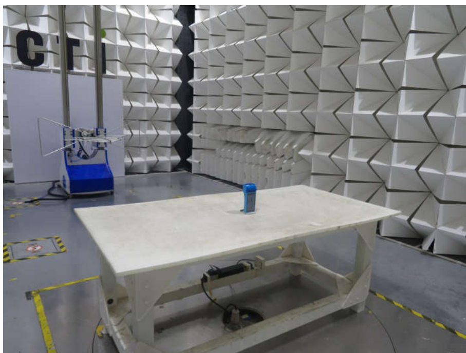
Radiated spurious emission Test Setup-2(Below 1G)
