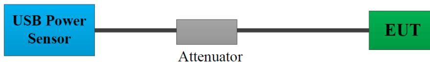
A short RF cable with low cable loss connected to the EUT antenna port, which was provided by manufacturer. The insert loss of this RF cable/attenuator was offset into the setting of test equipment.
