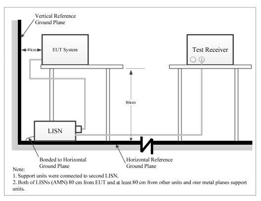
The setup of EUT is according with per ANSI C63.10-2013 measurement procedure. The specification used was with the FCC Part 15.207, RSS-Gen limits.
