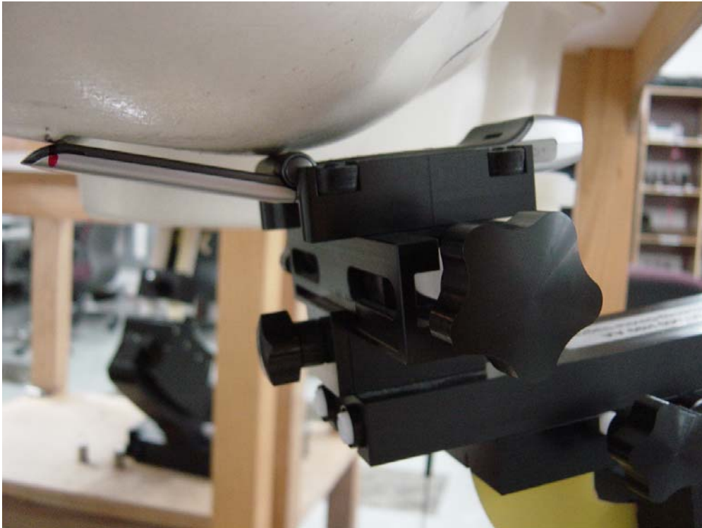
Figure 5. Phone Against the Head Phantom (Cheek Touch)
