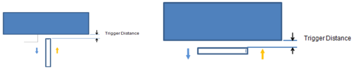
Picture: Proximity sensor triggering distances assessment (Bottom side) ..... Picture: Proximity sensor triggering distances assessment (Back side)
