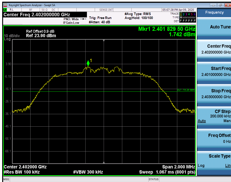
RF Conducted Spurious Emissions_2DH5_2402
