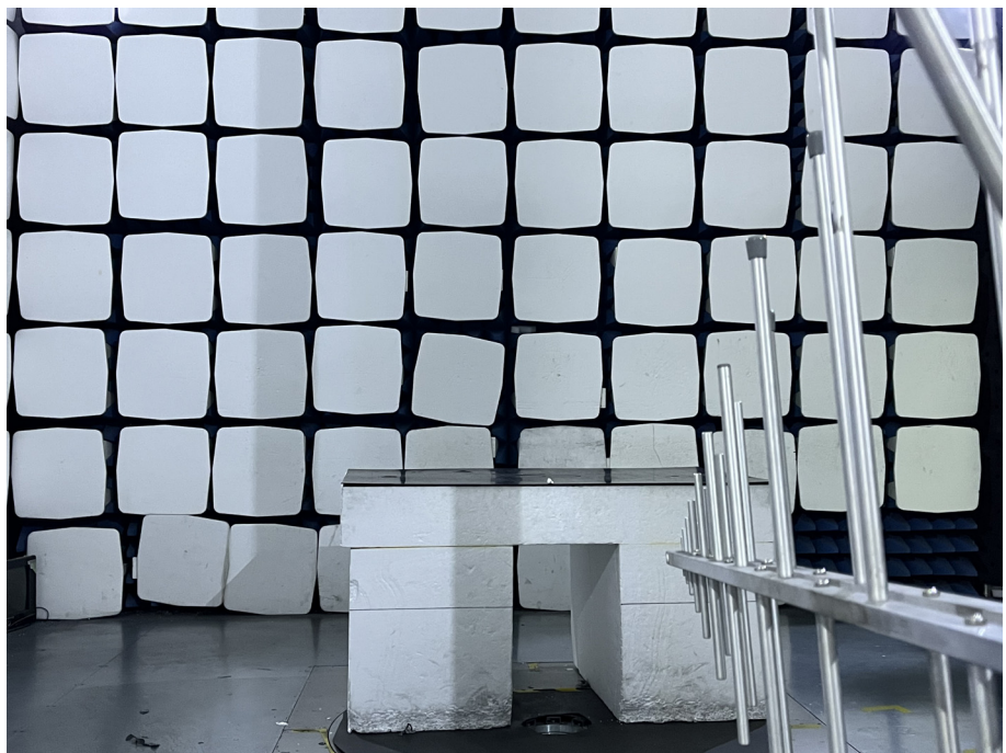
Radiation Emission Test Setup (30MHz to 1GHz)
