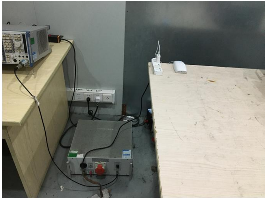
Conducted Emission Test Setup
