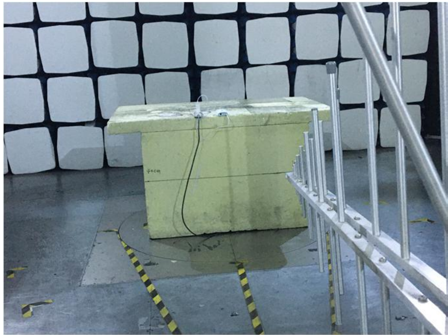
Radiation Emission Test Setup (30MHz to 1GHz)
