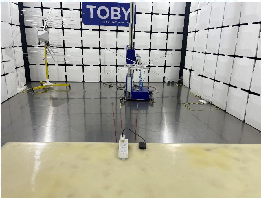
Photo of Setup for Radiated Emission (30MHz~1GHz)
