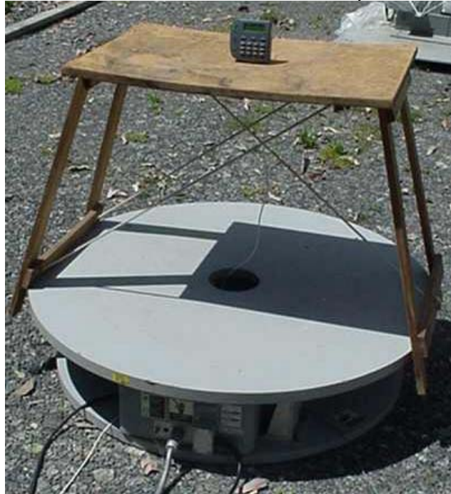
Radiated emissions test set up
