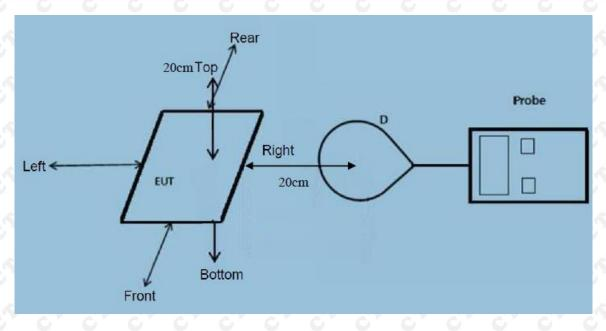
Note: Measurements should be made from all sides and the top of the primary/client pair, with the 20 cm measured from the center of the probe(s) to the edge of the device
