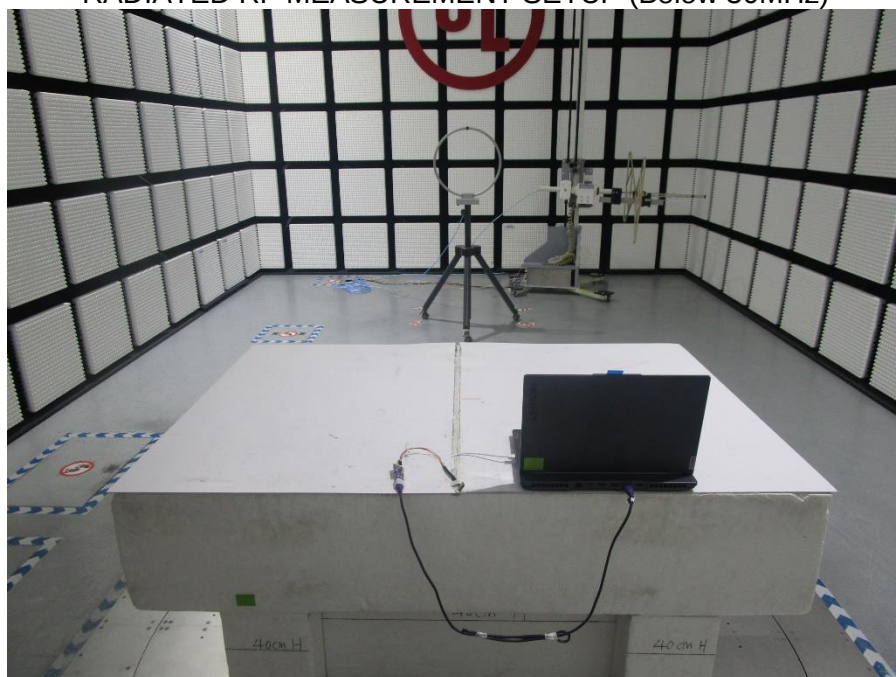
RADIATED RF MEASUREMENT SETUP (Below 30MHz)
