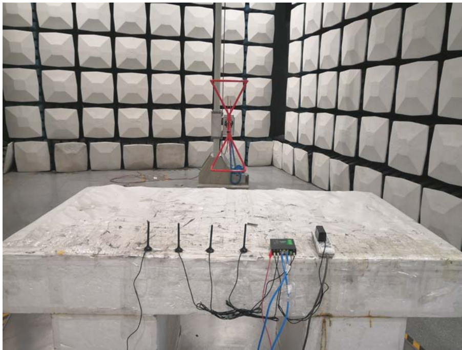
Radiated Emission Rear View (Below 1GHz)
