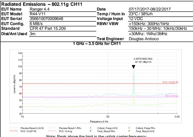
Note: Peak above the limit is the uplink carrier frequency.
