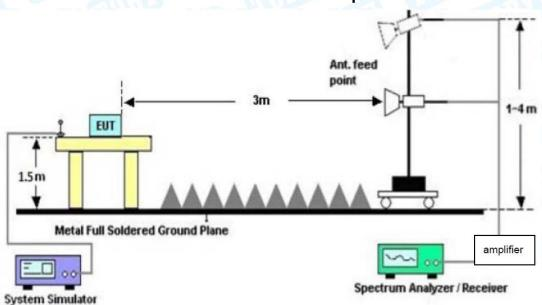
**Above 1GHz Test Setup**
