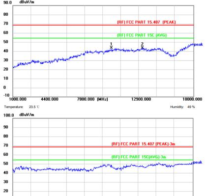
Level Limit Frequency Reading Factor Margin No. Detector (dBuV/m) (dBuV/m) (MHz) (dBuV) (dB/m) (dB) 1 \* 45.22 10282.000 -1.6043.62 68.30 -24.68peak 2 41.66 1.92 13189.000 43.58 68.30 -24.72peak
