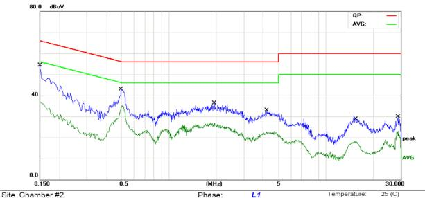
Limit: FCC Part 15B Class B Conduction(QP)
