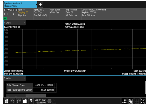
N5(10M)_DFT-s- OFDM_QPSK_Edge_1RB_Left_Low_CH_CHP_PA SS
