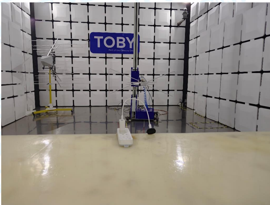
Photo of Setup for Radiated Emission (30MHz~1GHz)
