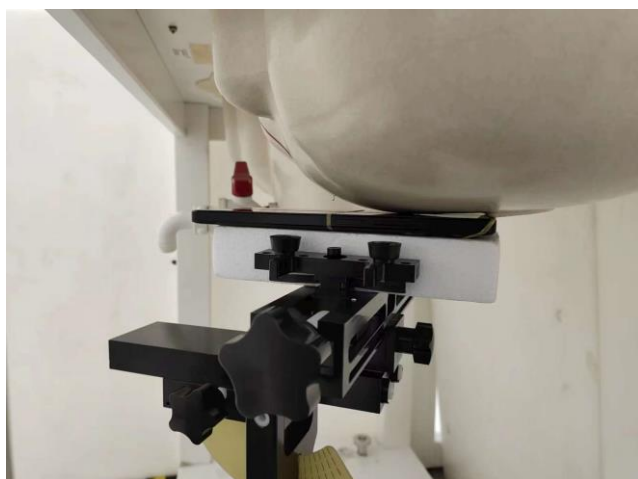
Left Cheek, Test Separation 0 mm
