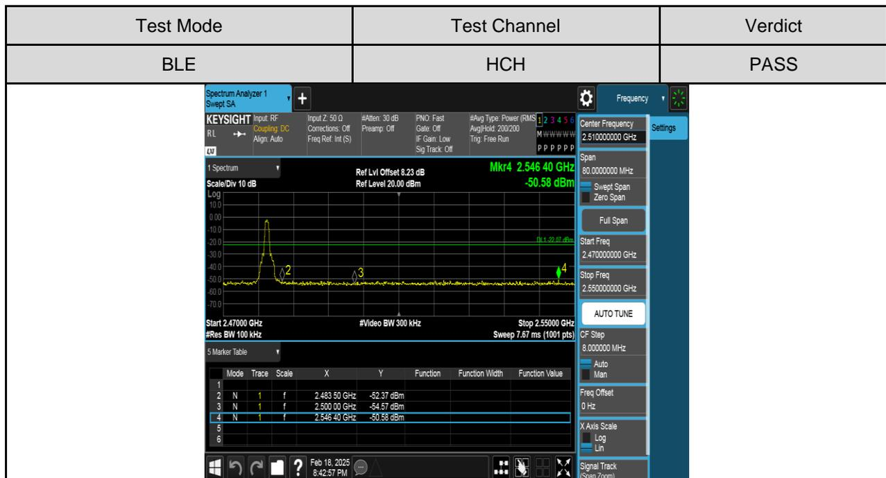
**PART 3: CONDUCTED SPURIOUS EMISSION****TEST RESULTS TABLE**
