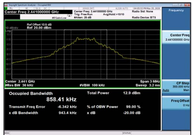
20dB Bandwidth: DQPSK,2402MHz,2DH5
