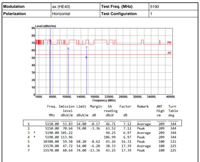
Note 1: Emission Level (dBuV/m) = SA Reading (dBuV/m) + Factor\* (dB)
