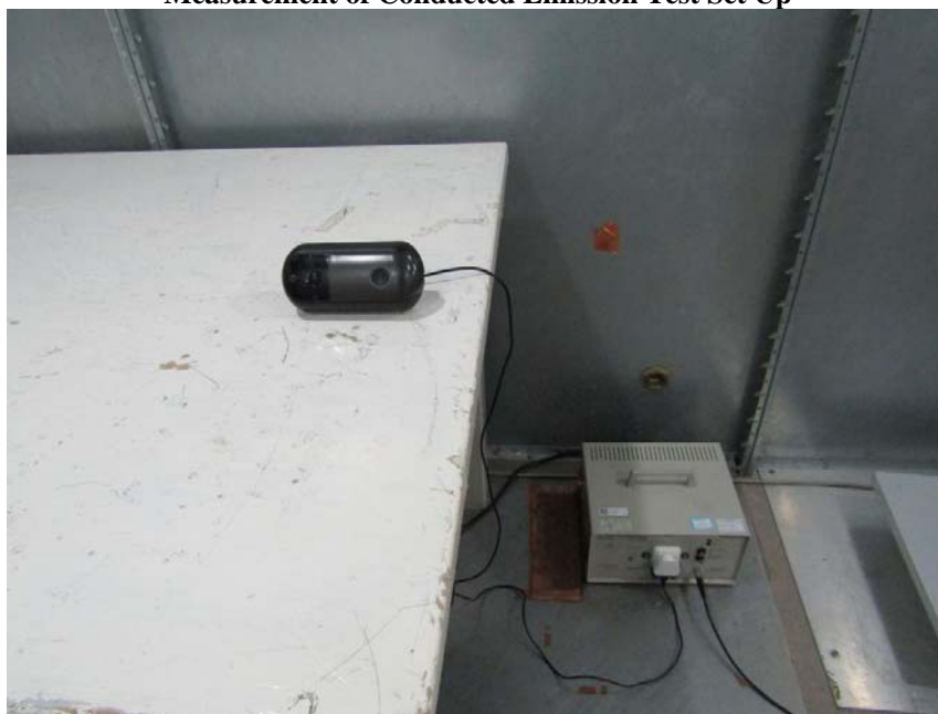
Measurement of Conducted Emission Test Set Up
