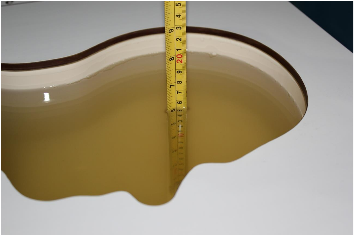
Picture 7-11: Liquid depth in the Head Phantom(2550MHz)
