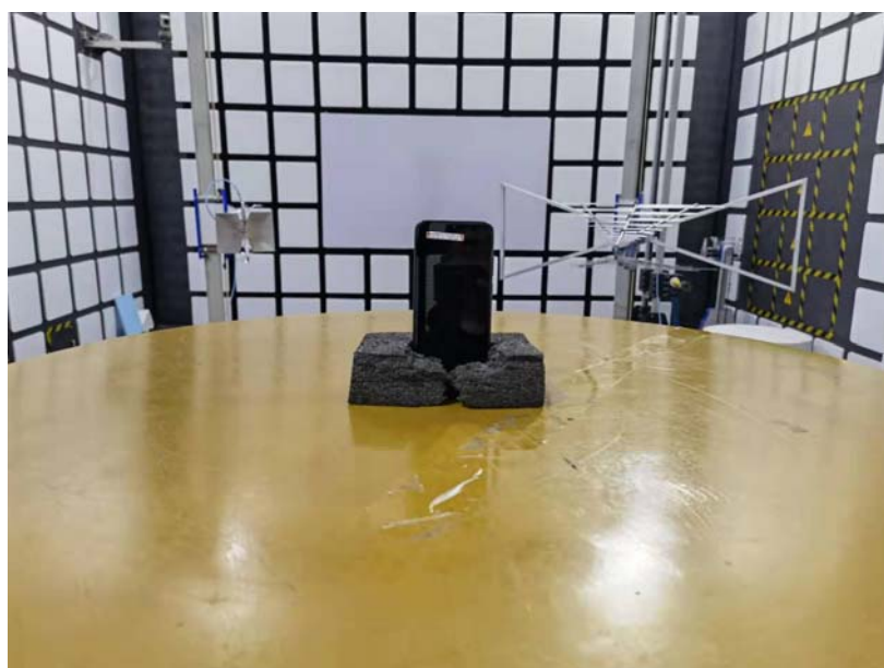
Spurious Radiated Emissions Test setup
