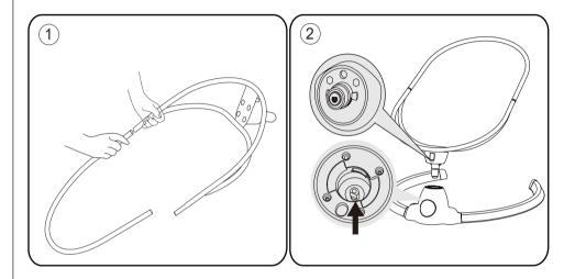
3. Wrap the seat cushion around the seat frame and secure the lock.
