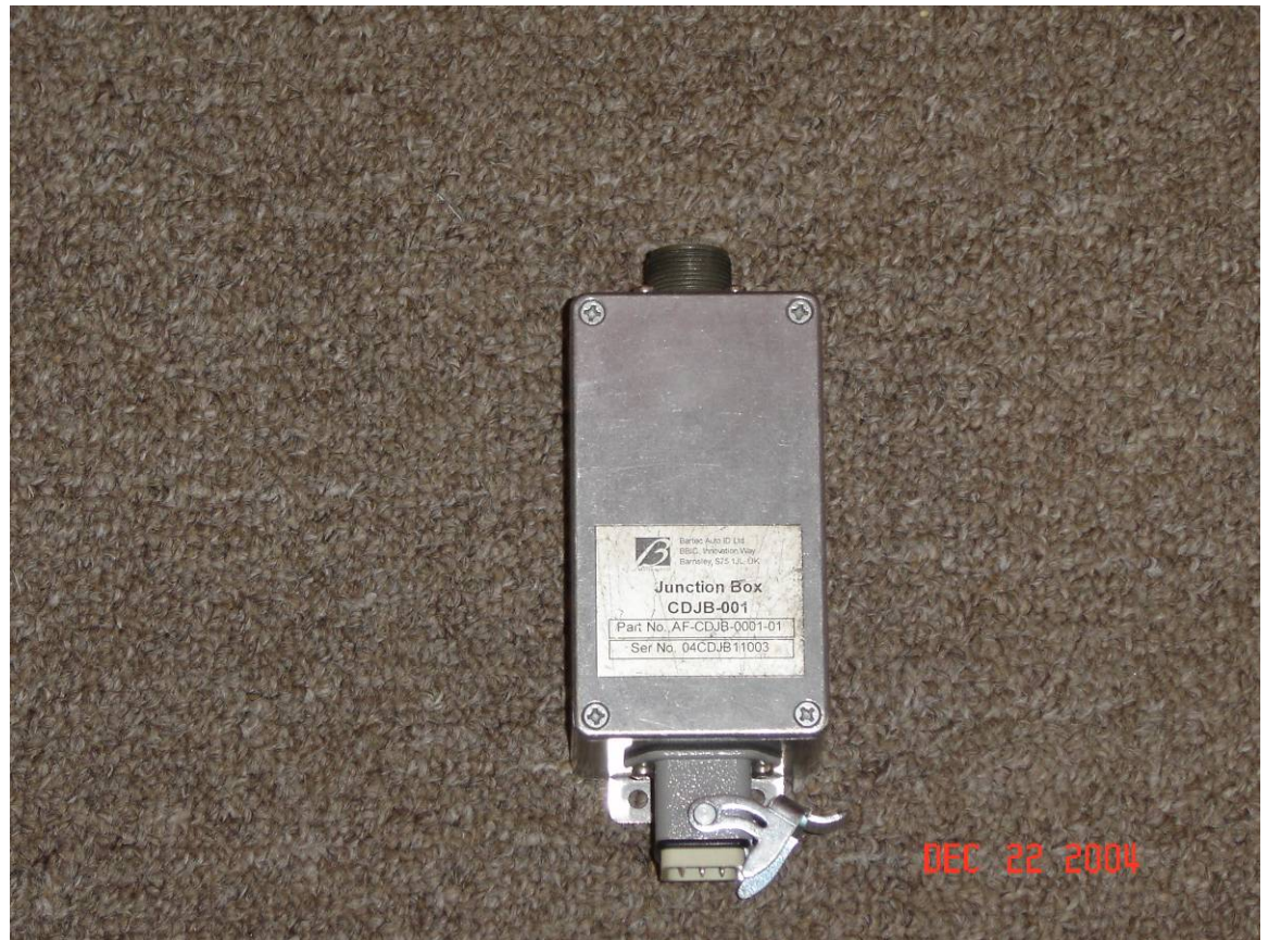
110 VOLT JUNCTION BOX (part no. AF-CDJB-0001-01)
