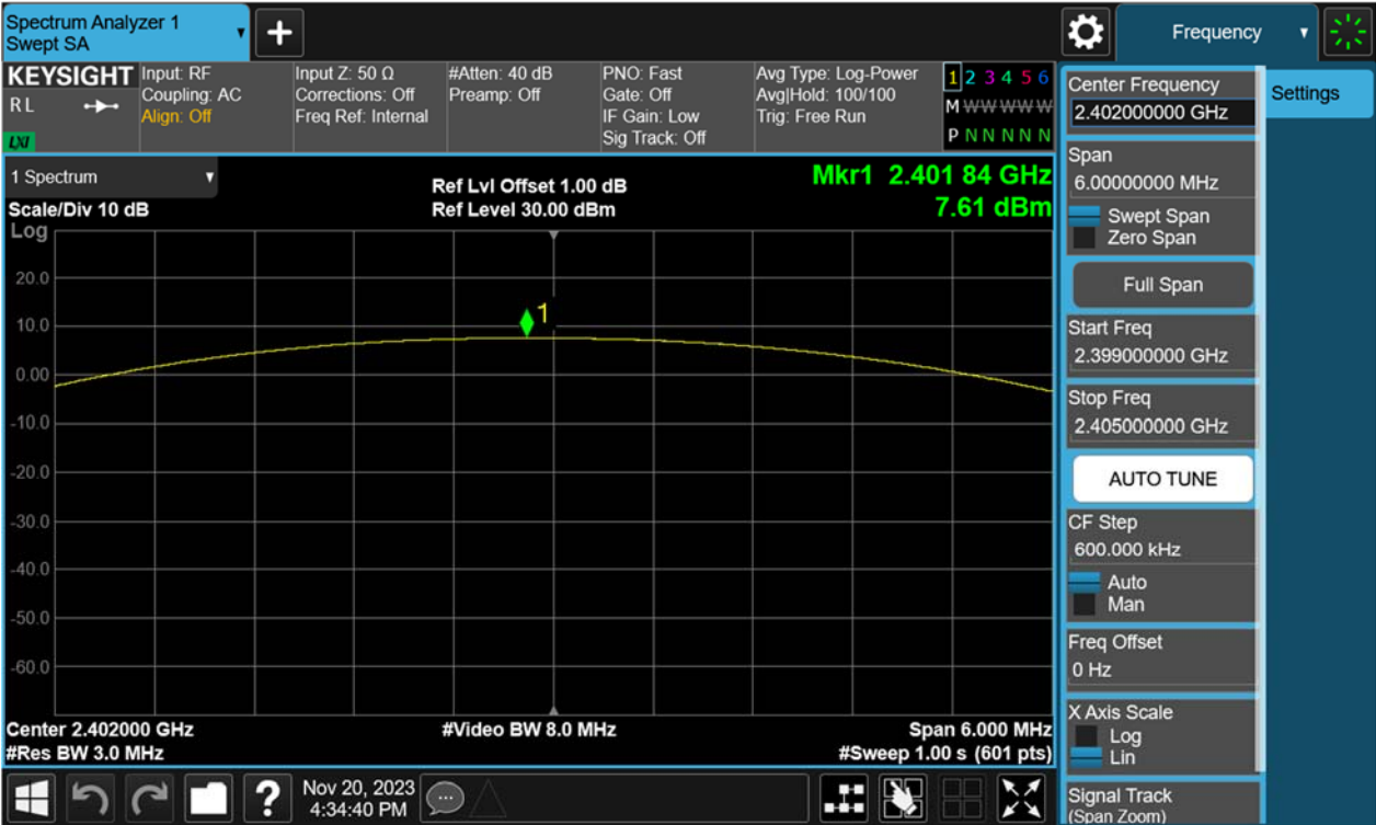
Figure 4: Maximum Peak Output Power, 2402MHz, \pi/4 -DQPSK
