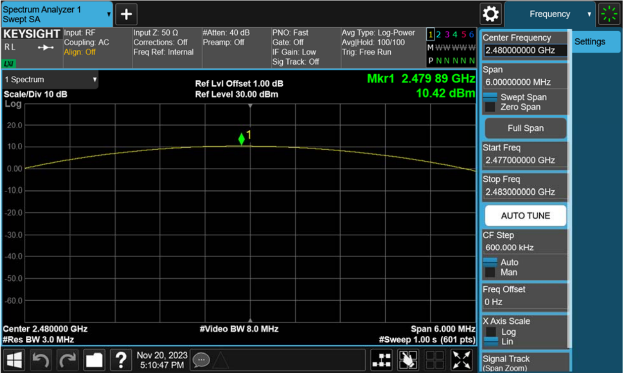
Figure 9: Maximum Peak Output Power, 2480MHz, 8-DPSK
