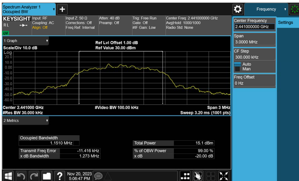
Figure 17: 20dB Bandwidth and 99% Bandwidth, 2441MHz, 8-DPSK
