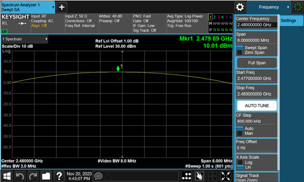
Figure 6: Maximum Peak Output Power, 2480MHz, \pi/4 -DQPSK
