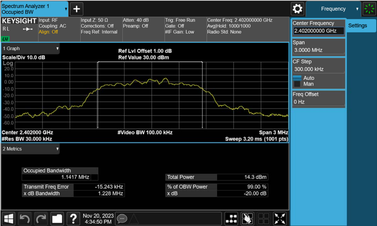
Figure 13: 20dB Bandwidth and 99% Bandwidth, 2402MHz, \pi /4-DQPSK
