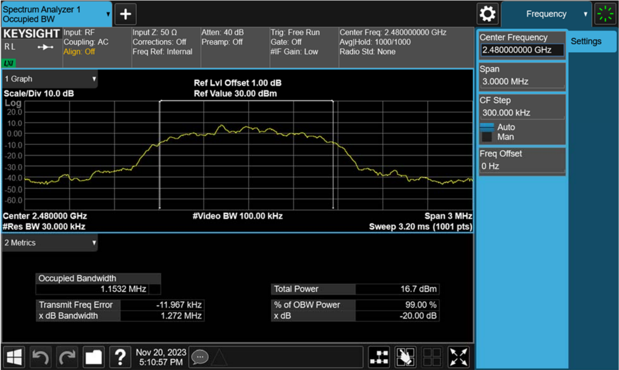
Figure 18: 20dB Bandwidth and 99% Bandwidth, 2480MHz, 8-DPSK
