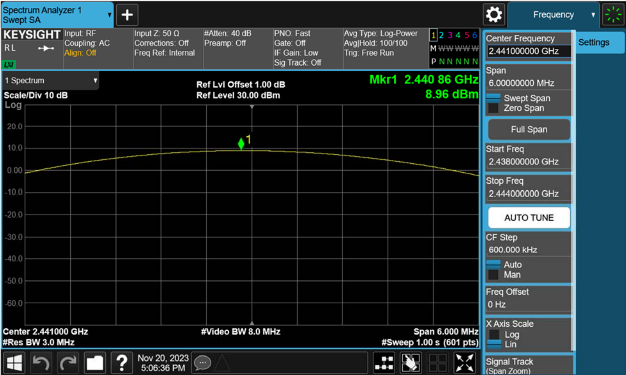
Figure 8: Maximum Peak Output Power, 2441MHz, 8-DPSK
