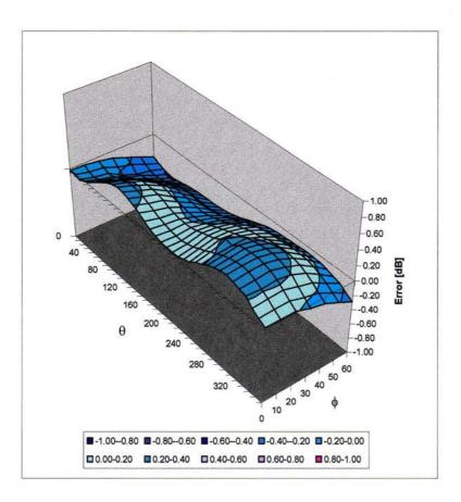
Spherical Isotropy Error < ± 0.4 dB
