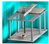
Figure 4-3 RF Near-Field Scanner
