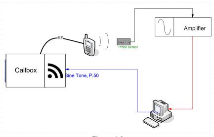
Figure 4-2 T-Coil Test Setup
