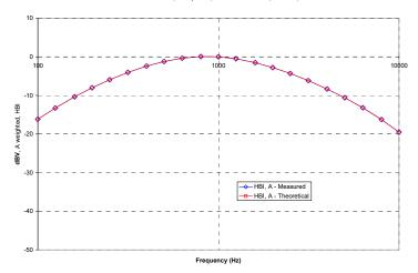
Figure 4-8 **ABM2 Frequency Response Validation**
