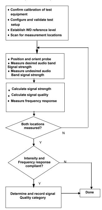
Figure 4-15 C63.19 T-Coil Signal Test Process
