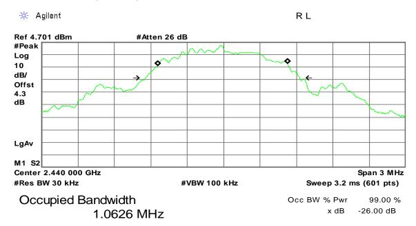
Transmit Freq Error -7.445 kHz x dB Bandwidth 1.273 MHz
