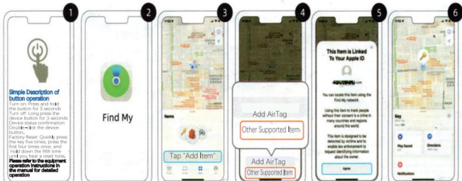
Press and hold the button for 3s to power on
