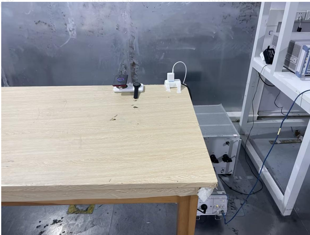
Conducted Emission-AC adapter charge mode
