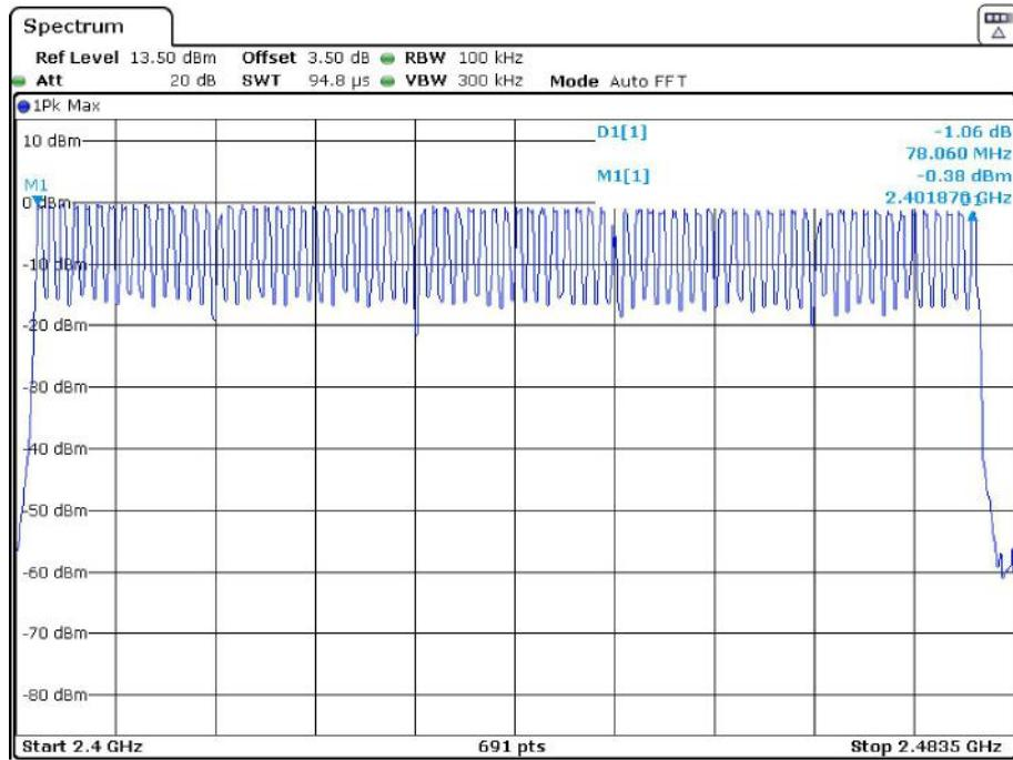
**EDR ( $\pi/4$ -DQPSK): Number of Hopping Channels**
