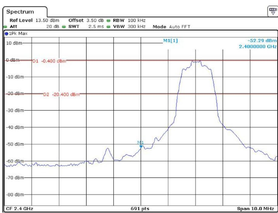
**EDR ( $\pi/4$ -DQPSK): Band Edge-Right Side****Hopping**
