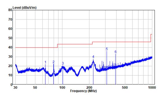
Site : chamber Condition: 3m Horizontal Job No. : SZNS211203-62353E-RF Test Mode: Charging+BT
