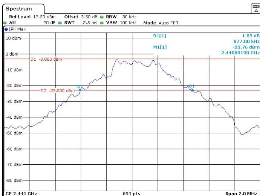
**BDR (GFSK): High Channel**
