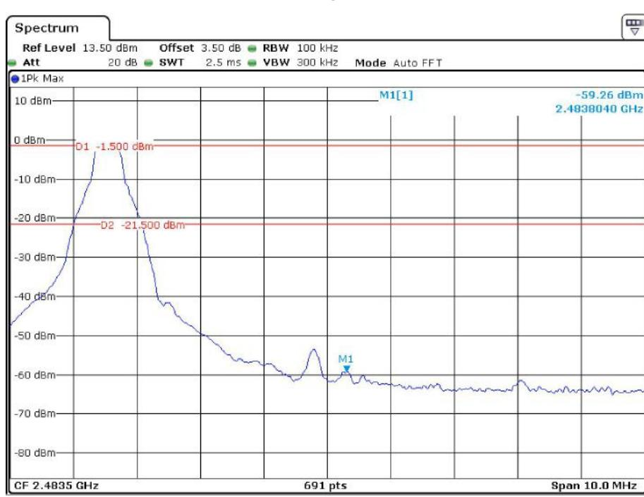
**EDR ( $\pi/4$ -DQPSK): Band Edge-Left Side****Hopping**
