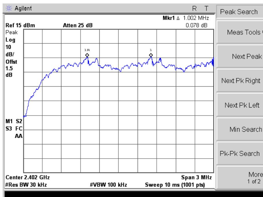
Channel Spacing (Middle CH=1MHz)
