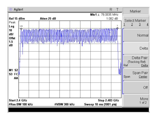
For GFSK mode Channel Spacing (Low CH=1MHz)
