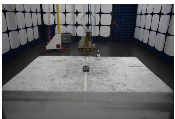
3. Radiated emission (9KHz-30MHz)
