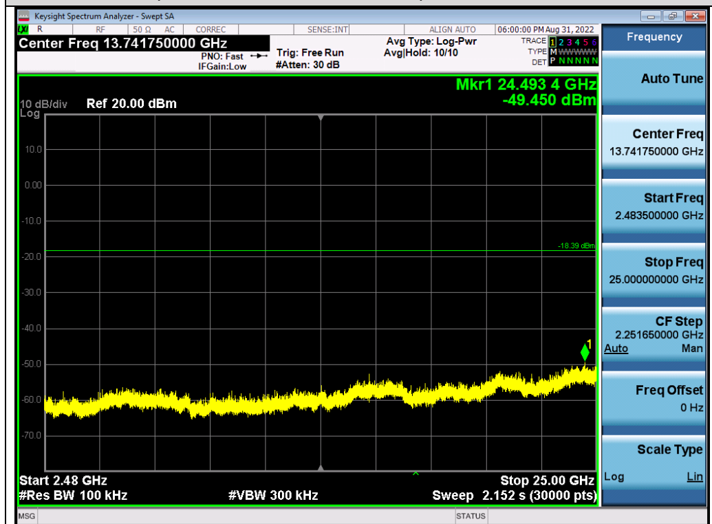
Test_Graph_802.11b_ANT1_2412_1Mbps_Higher Band Emissions
