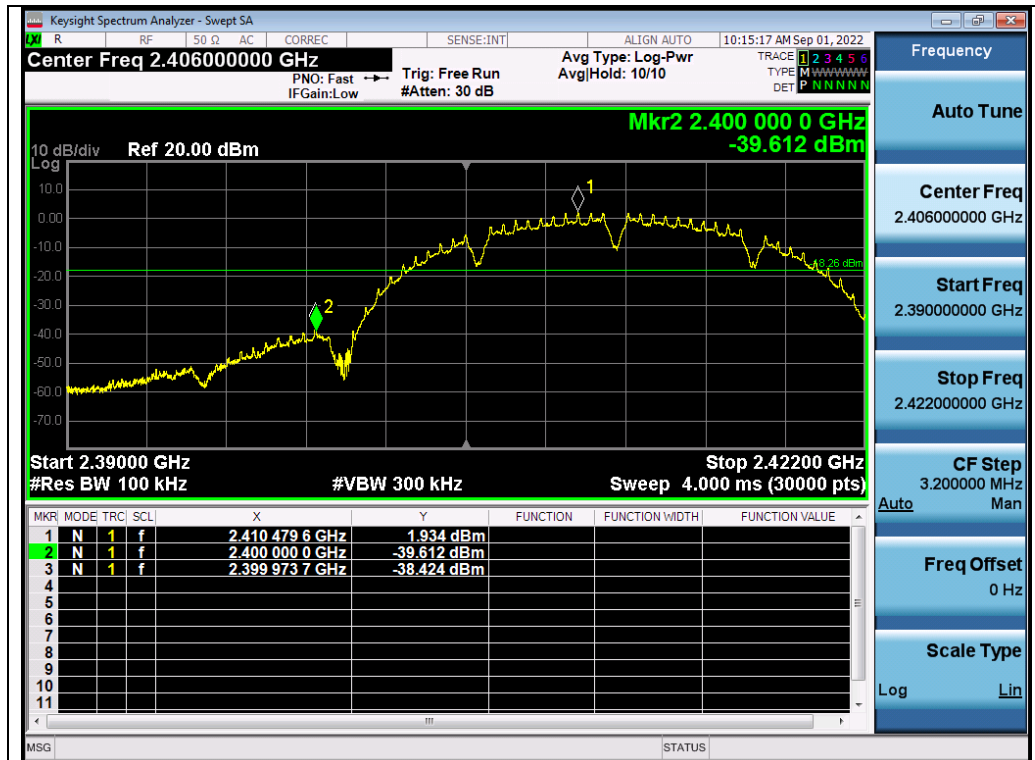
Test_Graph_802.11b_ANT1_2412_1Mbps_Lower Band Edge Emissions
