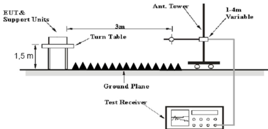
The radiated emission Below 1GHz tests were performed in the 10 meters chamber, above 1GHz tests were performed in the 3 meters chamber B, using the setup accordance with the ANSI C63.10-2013. The specification used was the FCC 15.209, and FCC 15.247 limits.
