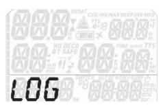
Quad 2 can record the profiles of over 100 hours of diving, at a sampling rate of 5 seconds. The information can be transferred to a Smartphone (Mares or MySSI app, via bluetooth). In addition, Quad 2 can show most of the information directly on the display. Upon entering the logbook you will see **StAt**. Entering this menu will show the
