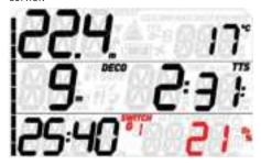
Use **BR-SP** while this indication is blinking to initiate the gas switch: the oxygen percentage of G2 starts to blink in lieu of that of G1, and in the top right corner the MOD of G2 is displayed, also blinking.
