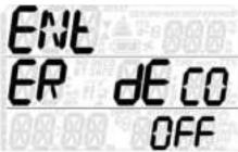
When this is set to ON, a warning will alert you when a mandatory decompression stop has been calculated by Quad 2.
