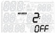
When this is set to ON, a warning will alert you when the NO STOP time reaches 2 minutes.
