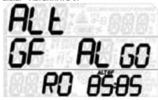
Quad 2 allows you to define an alternate set of gradient factors, to use when you need to cut your decompression short in case of an emergency. The set of alternate gradient factors cannot be more conservative (i.e. lower) than the main set of GF values. The default value is R0 (85/85).
