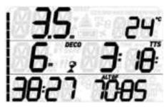
In this case, if the diver attempts a repetitive dive after surfacing, Quad 2 will function only as a depth gauge and timer (bottom timer mode) and it will display the missed deco stop violation symbol (2).
