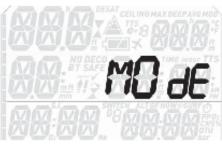
In this menu you define the type of gas you will be breathing during the dive (AIR as SINGLE GAS, NITROX as SINGLE GAS, NITROX as MULTIGAS). You can also set Quad 2 to BOTTOM TIMER, in which case Quad 2 will show only time, depth and temperature: it will not carry out any decompression calculation and it will not show any warnings and alarms.
