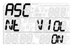
If the ascent rate exceeds 120% of the allowed value over a depth change of more than 20m/66ft, due to the potential of harmful bubble formation, Quad 2 locks the computer for 48 hours in order to prevent you from diving
