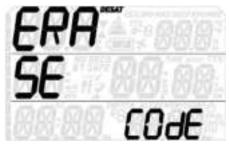
Quad 2 allows you to reset the desaturation in the computer. Any tissue saturation information from a recent dive will be reset to zero and the computer treats the next dive as a non-repetitive dive. This is useful when the computer is loaned to another diver who has not dived in the last 24 hours.
