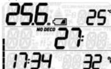
If the symbol starts blinking during a dive you must replace the battery before diving again.
