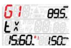
Quad 2 allows you to set up to 5 gases in which in addition to the oxygen percentage you can also set the helium percentage. Everything is the same as with multigas nitrox diving with the addition of OTUs (Oxygen Toxicity Units) in the sequence of data fields in the bottom right corner.
