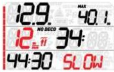
This persists until the ascent rate is reduced to below the pertinent limit. The limits are dependent on the current depth as follow:
