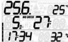
As soon as depth decreases Quad 2 activates the ascent rate control algorithm and displays the calculated value both numerically and graphically.
