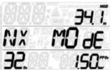
Once inside this menu, use TR-SP or BR-SP to change the  $0_2$ %, and watch how this affects the maximum operating depth (MOD). Then with TL-SP or TR-LP move on to the pp $0_2$ max and use TR-SP or BR-SP to change the value, again noticing how this affects the MOD. TL-SP or TR-LP saves the set values and returns to PRE-DIVE. Note that if you press BR-LP after setting the  $0_2$ % value, you skip the pp $0_2$ max setting and return directly to PRE-DIVE.
