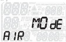
When selecting Nitrox, you can define the percentage of oxygen in the mixture  $\{0_2\%\}$  and the maximum value of oxygen partial pressure  $\{pp0_2max\}$  for up to three breathing mixes. The maximum possible value for the  $pp0_2max$  is 1.6bar. Most training agencies recommend not to exceed a value of 1.4bar.
