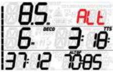
If the alternate gradient factors are not compatible with the current depth, Quad 2 considers this a dive violation and the deco violation symbol will appear, blinking, until you press any button to acknowledge having
