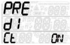
When set to **ON**, Quad 2 will consider all gases in the decompression calculation, with switches carried out at the MOD of each gas. When set to **OFF**, the decompression calculation will consider the currently breathed gas only. See Section 10 for more information about the **PREDICTIVE** feature.
