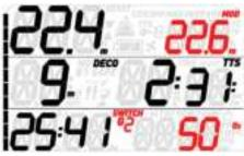
Use **BR-LP** to confirm the switch to G2: the set oxygen concentration will be displayed steadily in the lower right corner of the screen: if **PREDICTIVE** is set to **ON**, the decompression calculation will not change; if **PREDICTIVE** is set to **OFF**, within 20 seconds of having switched gas, the decompression calculation will be updated to reflect the change in gas.
