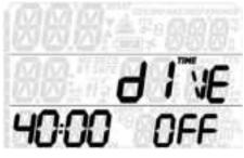
Quad 2 allows you to set a time alarm, triggering also a warning at half of the set time limit. The default value is OFF. Using the button, you can set the value between 20 and 90 minutes in 2-minute increments. Upon reaching half of the set limit, the dive time will blink until you hit any button to acknowledge it. Upon reaching the set time limit, the dive time again blinks until you hit any button to acknowledge it.
