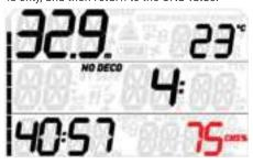
If the oxygen toxicity level reaches 75%, ascend to shallower depth to decrease oxygen loading and consider terminating the dive.
