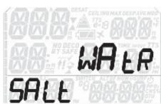
You can set the computer to fresh water, salt water or **EN13319** calibration, depending on where you intend to dive. Setting the wrong water type entails an error in depth measurement of maximum 3% (i.e. at a depth of 30m/100ft, a computer set to salt
