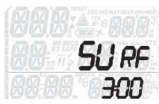
In this menu you can set the duration of the interval from the moment you reach the surface to when the dive computer closes the dive. During this interval you can submerge again and resume the dive. This menu allows you to change the default 3-minute interval to any value between 1 minute and 45 minutes.
