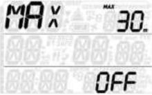
Quad 2 allows you to set an alarm at a depth independent of the MOD. The default value is OFF. Using TR-SP or BR-SP you can set it between 10m / 30ft and up to just shy of the MOD, in 1m / 5ft increments. Upon reaching the defined depth an alarm similar in behaviour to the MOD alarm (section 7.3.2) is triggered. Press any button to acknowledge having seen it.
