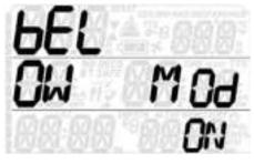
When set to **ON**, Quad 2 will allow a switch to a gas at a depth deeper than the MOD of the gas (resulting in an immediate MOD alarm).
